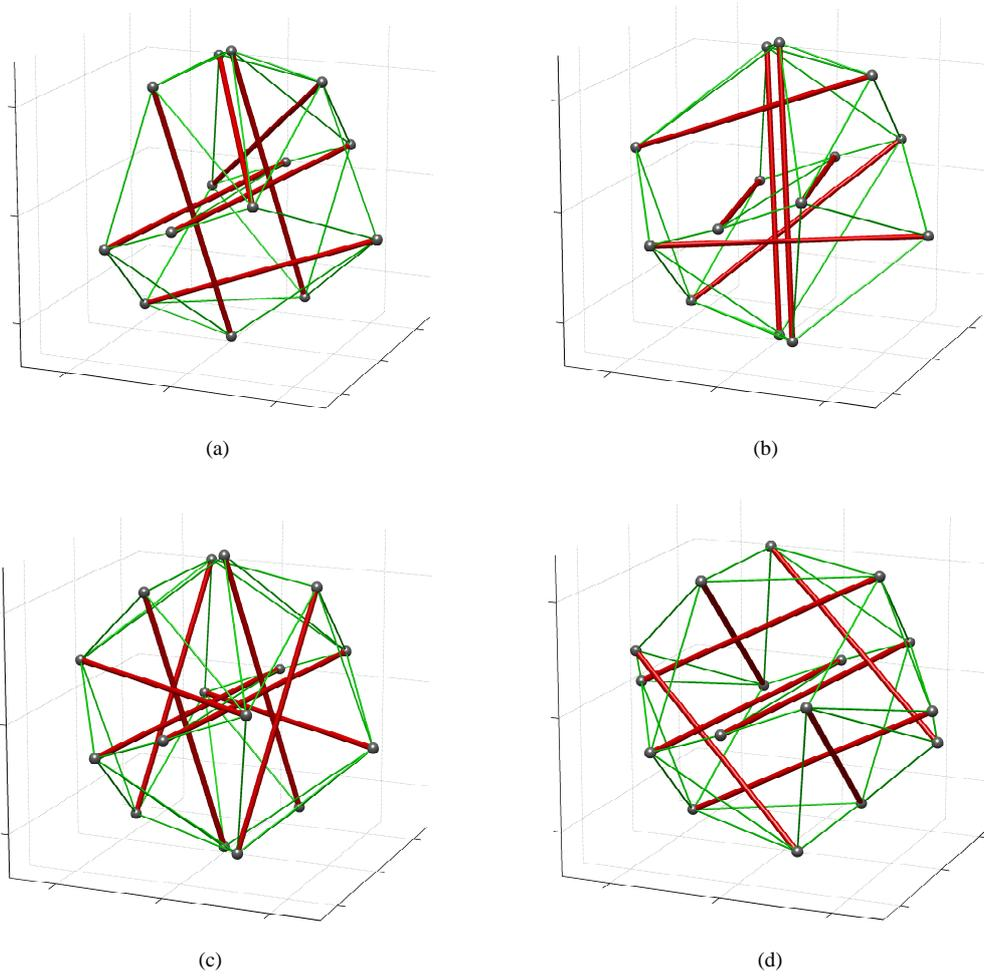
Fig. 3: Tensegrity structures with  $b_s = 3$  different strut lengths. (a)  $(s, b_s, b_c) = (7, 3, 5)$ ; (b)  $(s, b_s, b_c) = (7, 3, 6)$ ; (c)  $(s, b_s, b_c) = (8, 3, 4)$ ; and (d)  $(s, b_s, b_c) = (8, 3, 6)$ .
