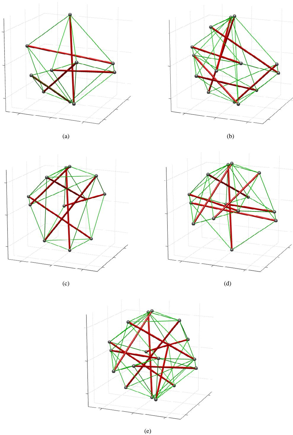
Fig. 5: Tensegrity structures with asymmetric configurations. (a)  $(s, b_s, b_c) = (5, 5, 8)$ ; (b)  $(s, b_s, b_c) = (5, 5, 18)$ ; (c)  $(s, b_s, b_c) = (6, 6, 9)$ ; (d)  $(s, b_s, b_c) = (7, 7, 10)$ ; and (e)  $(s, b_s, b_c) = (9, 9, 13)$ .
