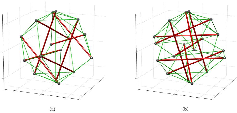
Fig. 4: Symmetric tensegrity structures with  $b_s = 4$  different strut lengths. (a)  $(s, b_s, b_c) = (8, 4, 5)$ ; and (b)  $(s, b_s, b_c) = (9, 4, 5)$ .
