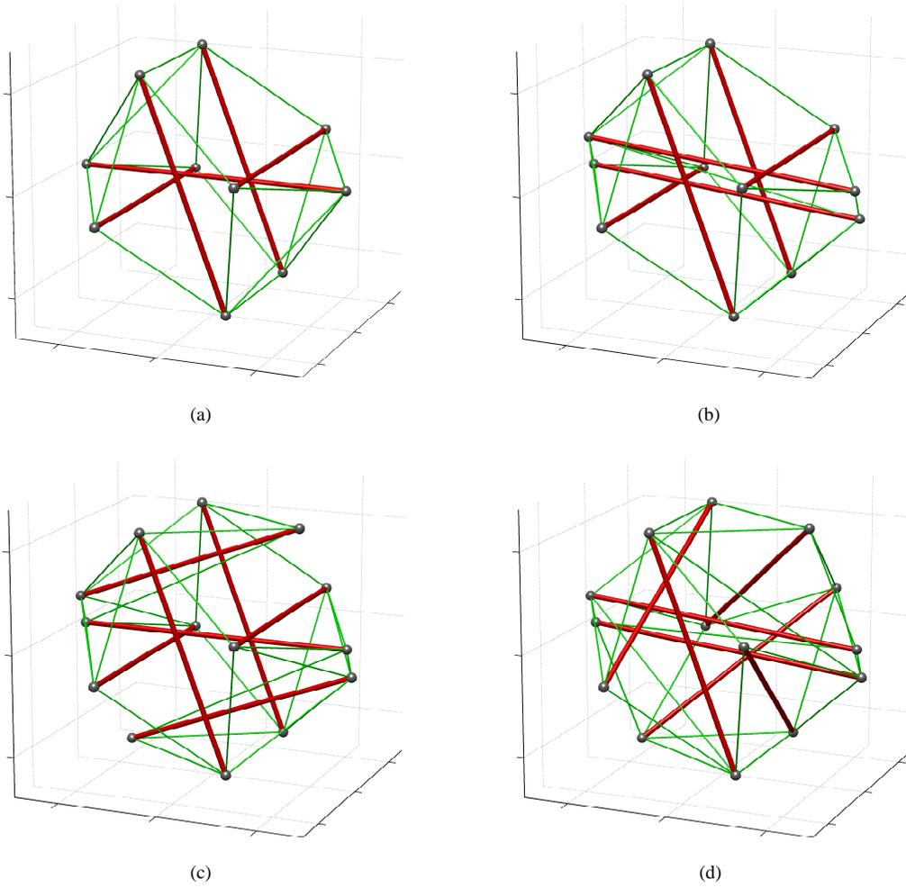
Fig. 2: Tensegrity structures with  $b_s = 2$  different strut lengths. (a)  $(s, b_s, b_c) = (5, 2, 3)$ ; (b)  $(s, b_s, b_c) = (6, 2, 4)$ ; (c)  $(s, b_s, b_c) = (7, 2, 4)$ ; and (d)  $(s, b_s, b_c) = (7, 2, 5)$ .
